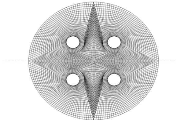
Figure 5 Free Surface Panel Model
