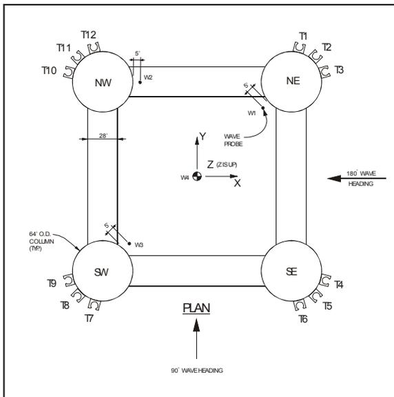
Figure 2 Wave Heading and Coordinate Definition
