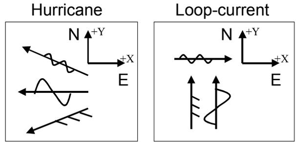
Figure 3 Wave, Wind and Current Directions in 100-year Hurricane WWC and 100-year Loop Current WWC
