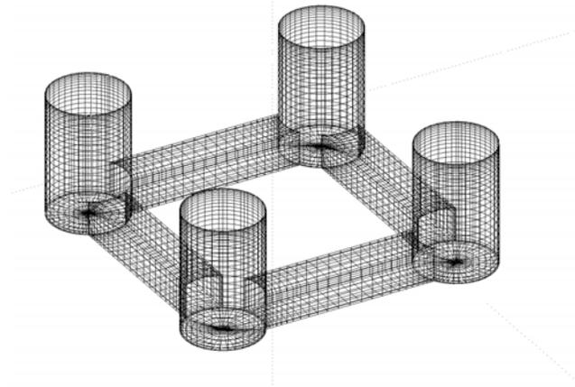
Figure 4 3-D Diffraction Hull Panel Model
